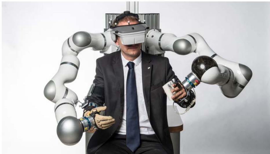
HUG – DLR’s bimanual haptic device [Hulin et al., ENACTIVE2008], [Hulin et al., ICRA2011]
