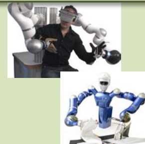
HUG – DLR’s bimanual haptic device [Hulin et al., ENACTIVE2008], [Hulin et al., ICRA2011]
