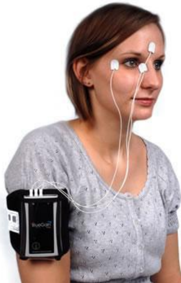
Figure 3 An EOG [17] device used to measure saccadic movements
