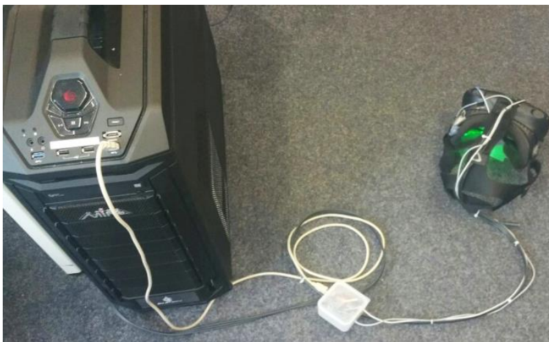
Figure 18 Experiment setup: PC, HTC Vive with an eye blink sensor and an LED turned on
