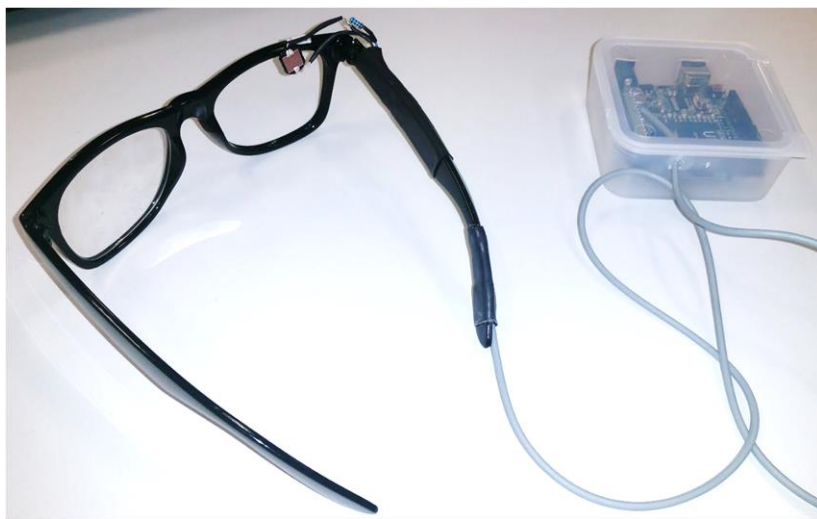
Figure 11 Universal sensor positioning device design based on eyeglasses to use in HMD
