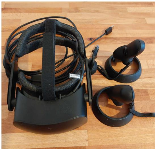
Figure 4.1: Picture showing the head-mounted display and controller (HP Reverb G2).
