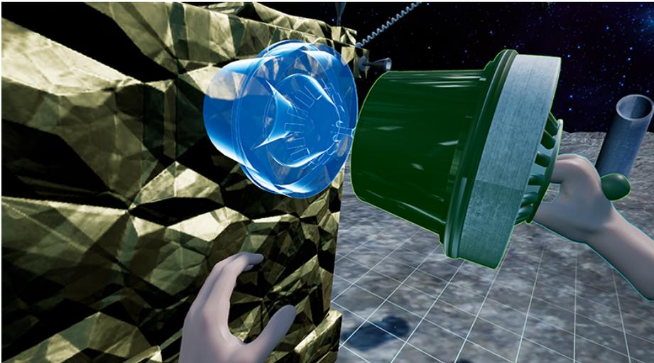
**Fig. 2** Bi-manual assembly in our virtual reality environment. The blue shaded part shows a projection of where the part will be mounted to, when released.
