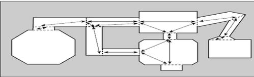
**Figure 12.8** The portals can be the nodes in a graph representing the map.
