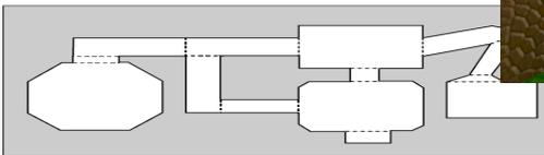
**Figure 12.7** Dotted lines represent the portals between convex areas.
