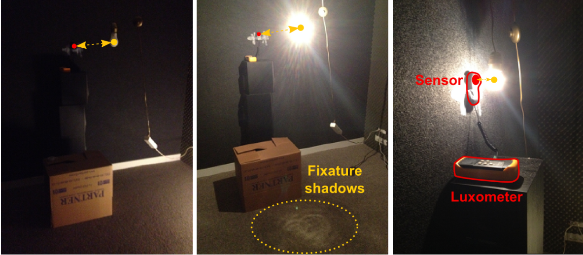
Figure 24: Lighting measurement setup: located in a sound room with no windows; walls are covered by a sound-reducing material with low albedo that reduces light bounce. The bottom right image shows that the light bulb was self-shadowing at the bottom, thus the intensity is not fully isotropic. Consequently, the measurement was taken horizontal to the filament. For each measurement, we waited a certain amount of time to let the light bulb warm up. Note that the incident meter is very sensitive to any obstructions (like a human body) or reflections (like a white surface). All measurements of distance are from the sensor of the incident light meter to the filament inside the light bulb.
