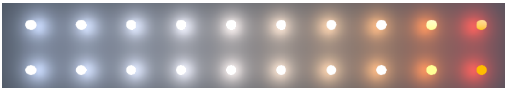
Figure 50: Example of emissive surfaces rendered in both forward (top) and deferred fashion (bottom). The spheres are all emissive objects and sphere area lights have been added at the same position as the emissive spheres.
