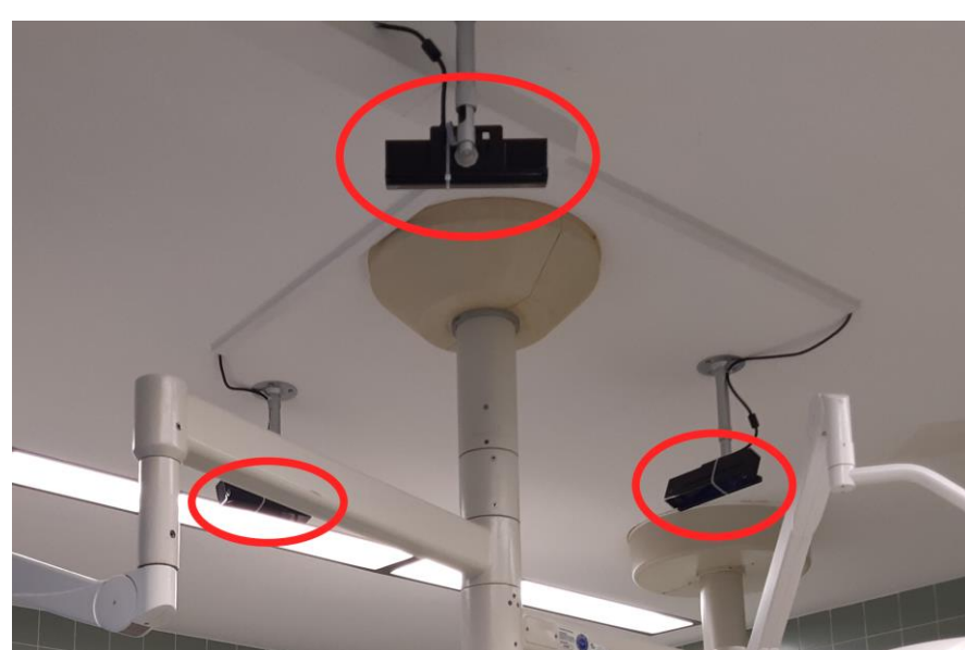
Figure 1. Depth sensors mounted on the ceiling of an operating room at the PIUS Hospital, Oldenburg, Germany.
