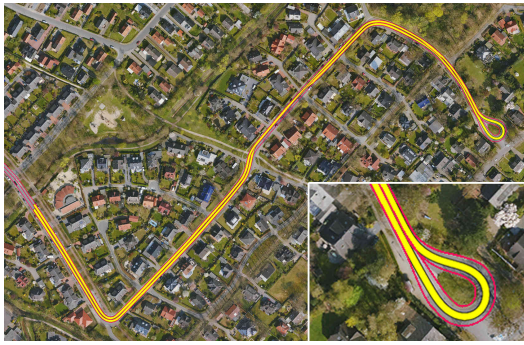
Fig. 9. © GeoBasis-DE / Landesamt GeoInformation Bremen 2019. Driven route (yellow) overlaid with the lanes (red) provided by the strategic decision making. The route starts in the east and leads to a turning circle to the west. After passing through it, the route returns to the starting point.
