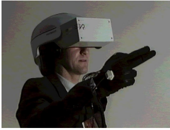
Figure 2: Some of the VR devices used at Fraunhofer IGD, roughly arranged from left to right according to their acquisition: a) VPL dataglove, Polhemus tracking sensor, and Virtual Research's Flight Helmet, b) Cyberglove and VR4 head-mounted display, c) Steward motion platform,
