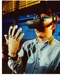
Figure 2: Some of the VR devices used at Fraunhofer IGD, roughly arranged from left to right according to their acquisition: a) VPL dataglove, Polhemus tracking sensor, and Virtual Research's Flight Helmet, b) Cyberglove and VR4 head-mounted display, c) Steward motion platform,
