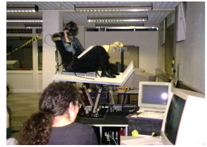
Figure 2: Some of the VR devices used at Fraunhofer IGD, roughly arranged from left to right according to their acquisition: a) VPL dataglove, Polhemus tracking sensor, and Virtual Research's Flight Helmet, b) Cyberglove and VR4 head-mounted display, c) Steward motion platform,
