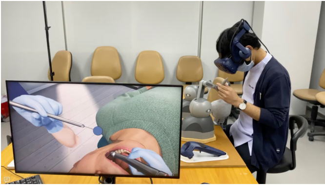
Fig. 1. The VR dental surgery simulator is used by a dentistry student to practice root canal access opening on tooth #36. The VR HMD and haptic input/output devices allow for an intuitive control with realistic haptic feedback (in alignment condition). The monitor shows the image that the student is seeing on the HMD.
