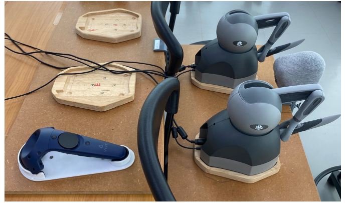
Fig. 2. The calibration of the haptic devices with the HTC Vive VR system is implemented using a VR controller with a static offset. The “hand-tool misalignment” is achieved by calibrating and then moving the haptic devices forward and downward in front of the table, as shown here.
