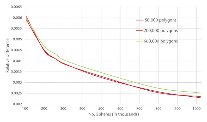
Accuracy of DPVI method w.r.t different resolution shape models of Itokawa
