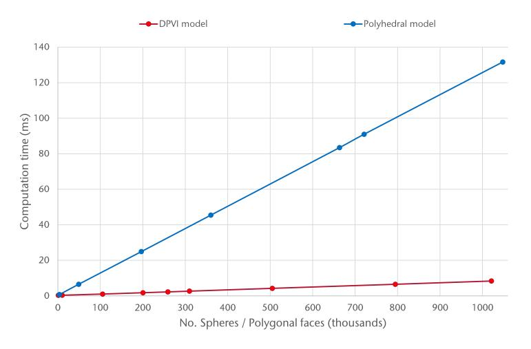
Time taken to compute acceleration at a given point
