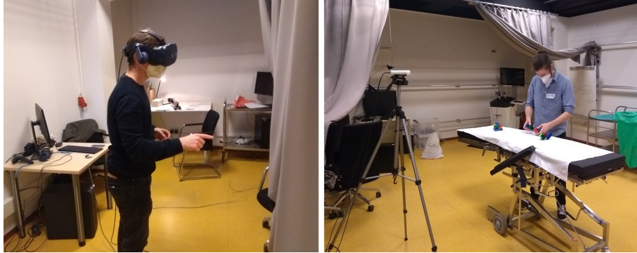
Fig. 6. Our telepresence system in action during the studies: on the left the remote doctor and on the right the live-captured operating room scene.
