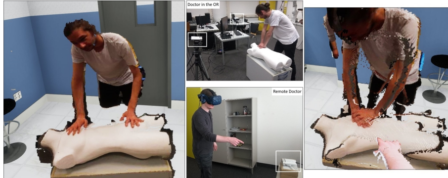
Fig. 2. Example of our system. Left: Live-streamed point cloud visualization of the local doctor in the real OR, seen from the perspective of a remote doctor. Middle: Physical environments of the local (top) and remote (bottom) doctors with RGB-D cameras (see white rectangles). Right: Point cloud visualization of the local doctor using two cameras to minimize occlusions, and part of the remote doctor’s self-avatar.
