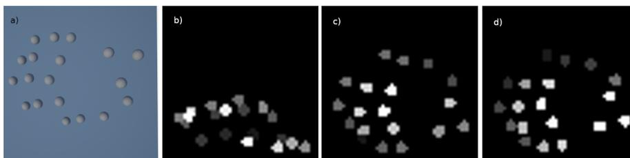
**Fig. 2.** Image a) shows the point cloud data of the tracked markers for a flat hand pose (small joint angles). To label the 3D positional data, a depth image is created from a). In b), the depth image was created from a random projection direction. Image c) uses a projection axis generated with the PCA method. Image d) was created using a projection axis perpendicular to the palm (PalmP). The depth information is visualized as pixel intensities.
