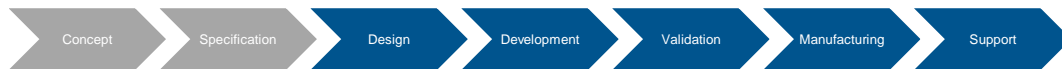
Figure 74 - Typical steps within automotive product lifecycle management. Those steps which can draw most benefit from the function-oriented 3D methods are highlighted in blue.
