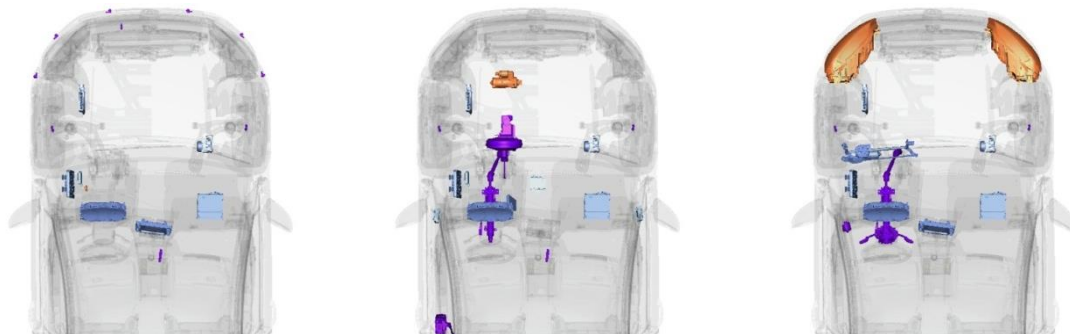
Figure 50 - The proposed methodology enables spatial comparison of multiple function architectures in specific vehicle projects. Left: park assist, middle: start stop, right: dynamic light assist
