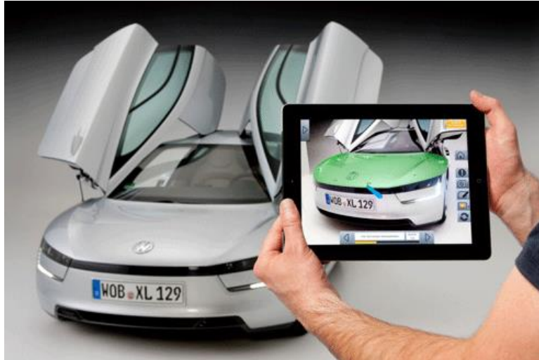
Figure 6 - Augmented reality example showing virtual data (color variant) being projected onto a physical car front end [36]
