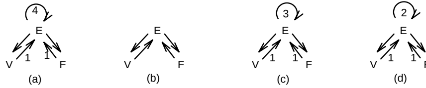
Figure 4.3. The winged-edge (a), complete vertex and edge list (b), quad-edge (c), and doubly-connected edge list (d), depicted by the relations they store.
