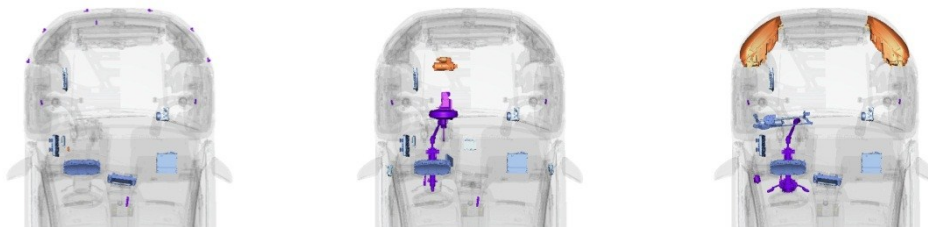
Fig. 8: Our work enables a spatial comparison of function architectures in particular vehicle projects. The example shows related components of the following functions (from left to right): (a) Park Assist , (b) Start-Stop Automatic and (c) Dynamic Light Assist .
