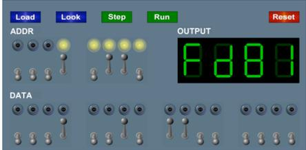
The image shows the front panel of the TOY computer. It features four buttons at the top: 'Load' (blue), 'Look' (blue), 'Step' (green), and 'Run' (green), along with a 'Reset' button (red). Below these are two rows of switches. The top row is labeled 'ADDR' and has 8 switches, with the first three illuminated. The bottom row is labeled 'DATA' and has 16 switches. To the right of the switches is a green 7-segment display labeled 'OUTPUT' showing the number '8888'.
