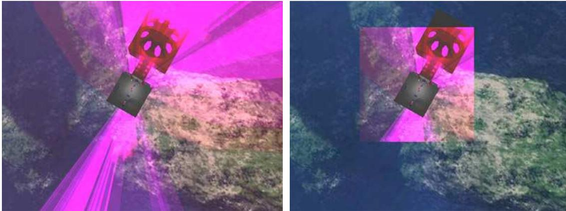
**Image 4.** *Left:* Top-view of the scene, with shadow volumes stretching to infinity despite the attenuated point light. *Right:* using the scissor region, we limit shadow volumes to the effective radius of the light and conserve fill rate.
