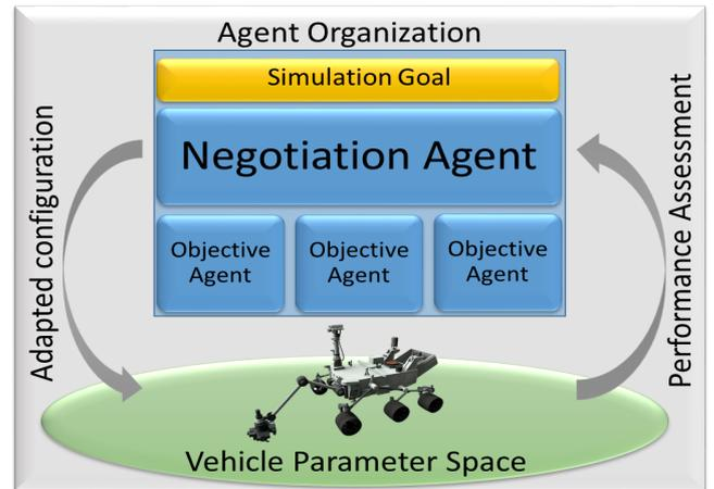
**Figure 4:** One agent organization is generated for each simulation goals. Each organization searches through the corresponding vehicle parameter space by measuring the vehicle performance and by adapting the configuration until the organization finds a satisfying solution.
