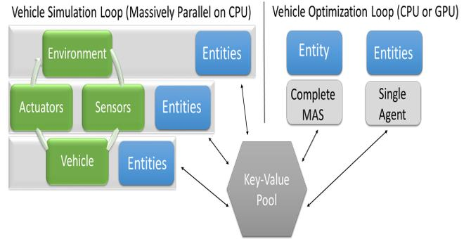
**Figure 3:** Entities are mapped to our generic vehicle simulation loop, consisting of the environment, sensors, actuators and internal vehicle components. Our MAS is either computed on the CPU with  $n$  Entities or on the GPU as one Entity with a single CUDA kernel for all agents.
