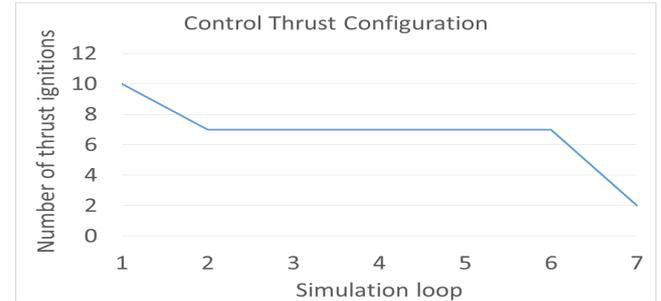
**Figure 13:** Our approach can gradually decrease the ignitions as the overall thrust level is increased by another agent.
