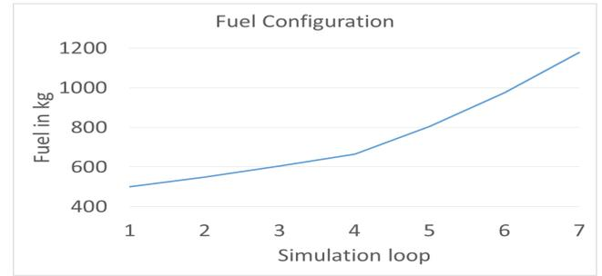
**Figure 12:** Our approach gradually increases the fuel capacity in order to maintain thrust while the landing procedure is conducted.
