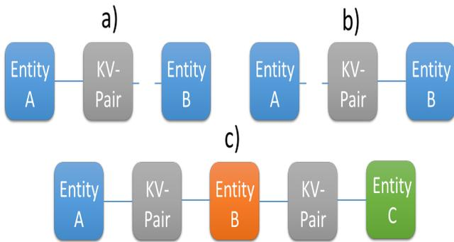
**Figure 6: Model validation for simulation data flow: a) If a key-value pair X is written by Entity A, at least one other Entity B must read it from the same graph b) If a key-value pair X is read by Entity B, it must be written by another Entity A from the same graph c) If data from Entity A should be perceived by Entity C which is not situated in the same graph as Entity A, it has to be transmitted by an interface Entity B.**
