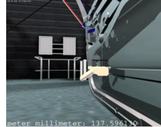
Fig. 11. With the virtual yard-stick distances can be measured in the VE.
