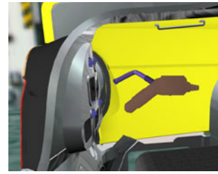
Fig. 17. Violations of security-distance are highlighted by yellow, collisions are red.
